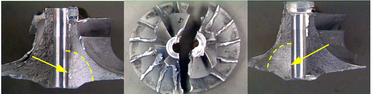
Figure 1: Classic type of LCF hub burst
